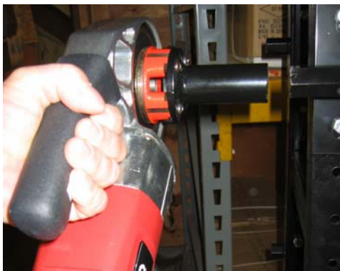
Slip onto core tube end. Try the winder prior to loading cover for first time.
