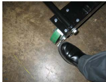
Lock brake PRIOR to loading cover
