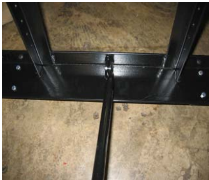
Attach cross brace to bottom center
