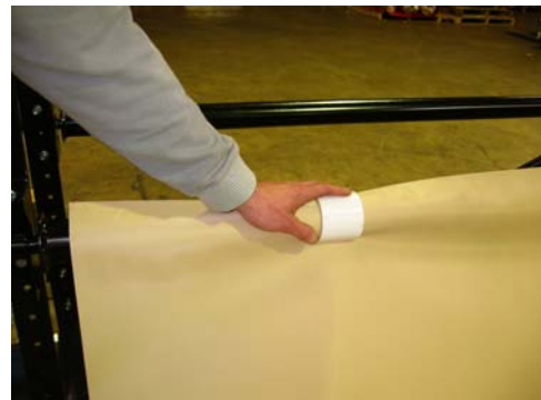
Place one clip retainer approx. 1/4 toward center from each end and one in center.
