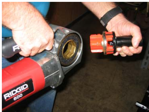
Adaptor fits onto power winder
